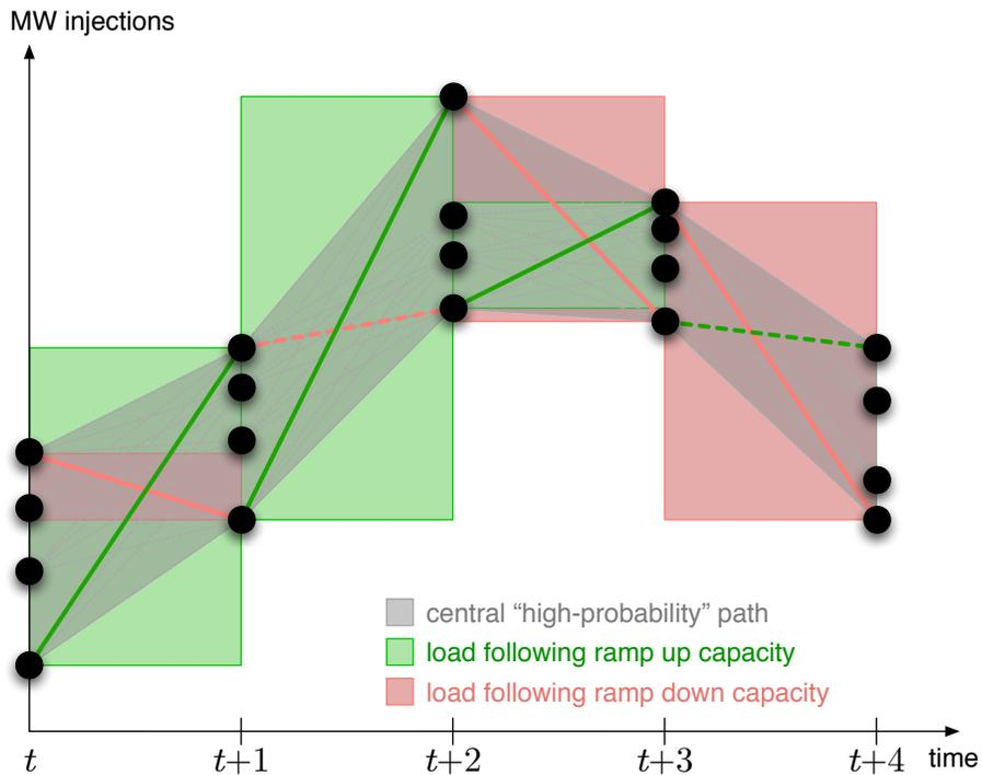
Figure 3-6: Ramping and Load Following Ramp Reserves
