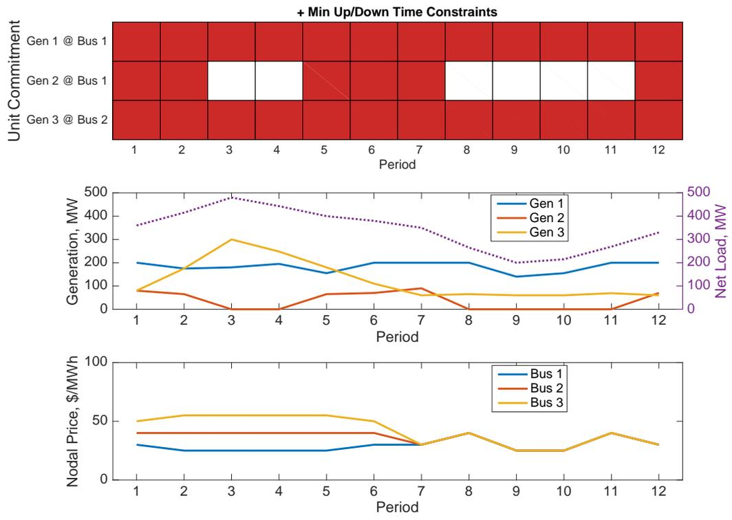
Figure 7-6: Deterministic UC : Add Min Up/Down Time Constraints
